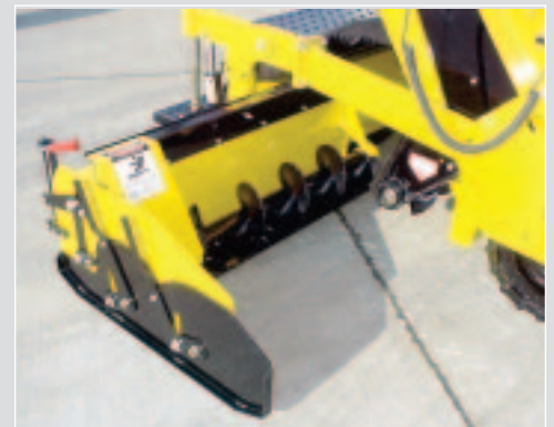
Full floating screed with (2) 30" hydraulically operated, adjustable screed extensions.
